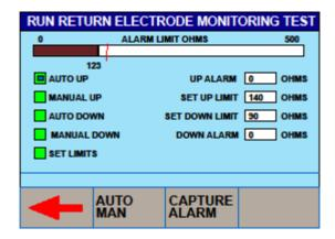
Select automatic (up or down) or manual (up or down) control by using the dedicated AUTO MAN key. This key is also used to set the limits. Once the SET LIMITS field is highlighted in green, use and press the rotary encoder to manipulate the UP and DOWN limits.
