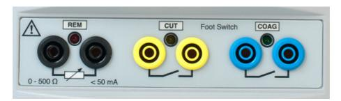
For automatic control during HF leakage and Power tests, connect the ESU footswitch COAG and CUT contacts to the blue and yellow terminals.
