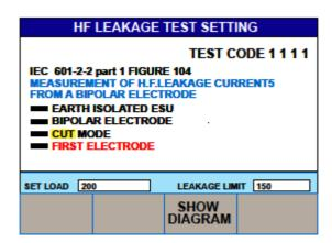
Press the rotary encoder to activate the SET LOAD and LEAKAGE LIMIT
