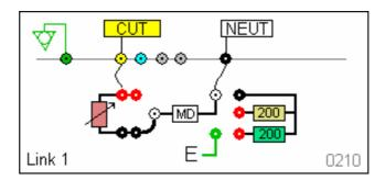
Connect the ESU active and neutral electrodes to the side panel as indicated, also fit jumper links (positions 1, 2, 3, 4) as required to complete circuits.
