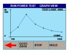
At the end of the test, toggle between GRAPH MODE and DATA by pressing the GOTO DATA fast key.
