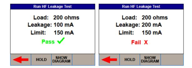
Press the HOLD key to freeze the reading on the screen.
