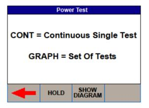
Select either the Continuous Single test (CONT) or GRAPH mode using the fast keys;
